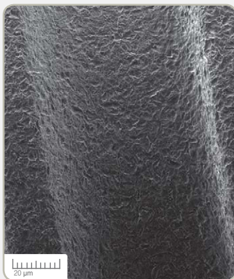
SEM image of the implant surface
